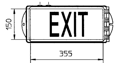
Emergency exit sign
