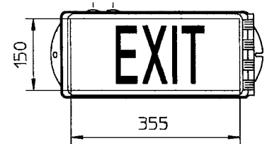
Emergency exit sign
